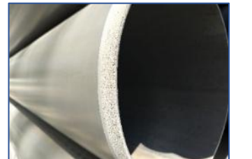
Wastewater pipes made of 100% recycled PVC
